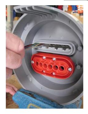
1. Secure the MFD by using a vise or a clamp
