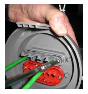
7. Fixate the outer part of the Window Cut port seal
