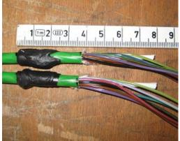
2. Make a window cut in the feeder cable
