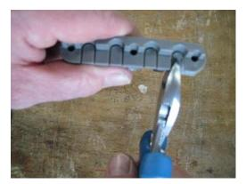
4. Break out the port(s) where a cable has been inserted
