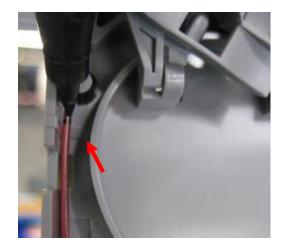
11. Strip the tubes from the markation point as shown in the picture
